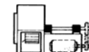
ARR. 9 SWSI. For belt drive. Impeller overhung. Two bearings with prime mover outside base.
