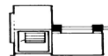
ARR. 1 SWSI. For belt drive or direct connection. Impeller overhung. Two bearings on base.
