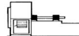
ARR. 4 SWSI. For direct drive. Impeller overhung on prime mover shaft. No bearings on fan. Prime mover base mounted or integrally directly connected.
